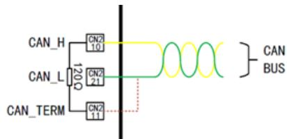
120Ω matching resistance: The factory default has this 120Ω matching resistance. If it is not needed, then cut the brown wire CAN\_ TERM (for multi-Communication purpose).
