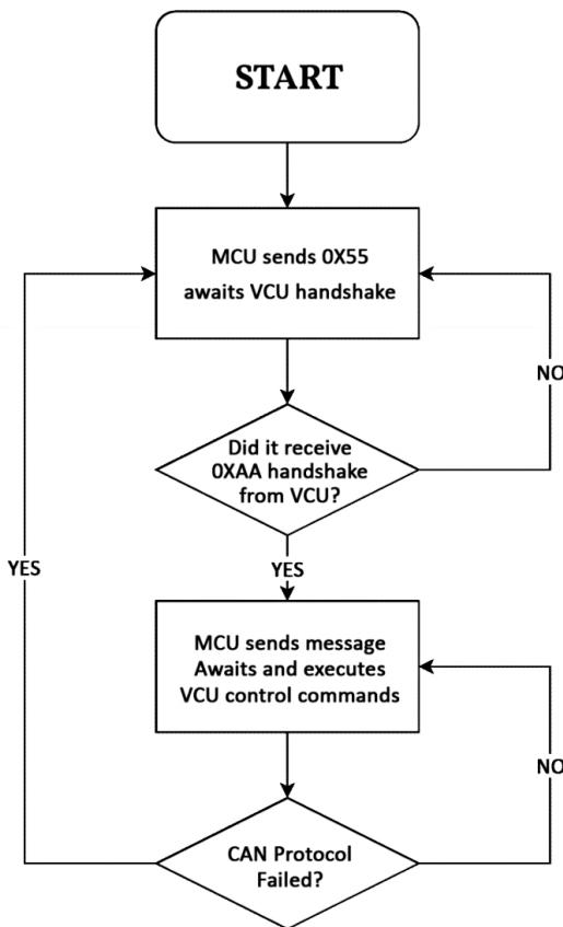
(1) The controller needs to do handshake first after it's powered on. After the handshake is successful, the controller will send the messages and receive the VCU control commands.
