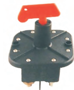
SF51622 Dual battery switch Used for dual battery system, Dual pole, studs: M10x2; M8x2 Type: on-off Max: 300A at 12Volts. Size: 90*90mm
