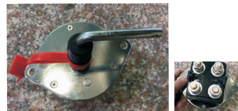
SF50632-2 Heavy duty battery switch Used for dual battery system, Dual pole ,12V-24V, 48V max Continue (Amp)200A, max 250A, Crank (Amp) 1000A, instant 2500A stud size: M10*4
