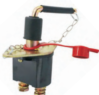
SF50632 Heavy duty battery switch 12V-24V, 48V max Continue (Amp)200A, max 250A, Crank (Amp) 1000A, instant 2500A stud size: M10*2
