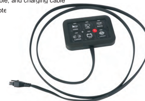
SF52117 12V Universal control panel Specification: Voltage: 12V, Max watt: 600W Switch panel: 6gang Relay: 40Ax6pcs Fuse: 30Ax1; 20Ax3, 15Ax2 Applicatin : Trucks/Rvs/Modified cars/Yachts/Jeep, etc
