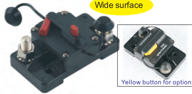
SF50650-31 20-150A wide surface breaker 1/4"-28 Studs SF50650-32 151-200A wide surface breaker 3/8"-16 Studs Wide surface mounting, manual on-off High-current waterproof circuit breaker
