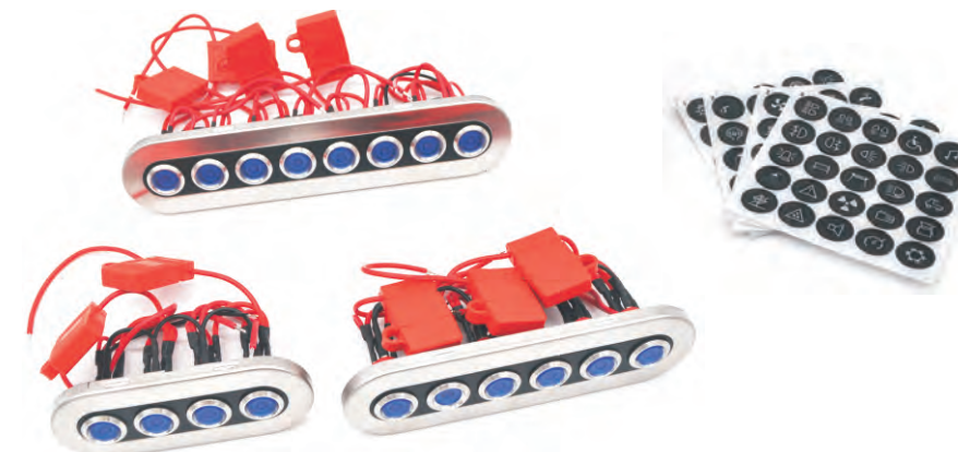
Waterproof Stainless Steel Button Switch panel Switch rating: 12V /24V 15A DC, IP65 Panel rating: Max. 20A per 2 branches Stainless steel &ABS panel, Stainless steel button switch including :labels stickers&mounting screws
