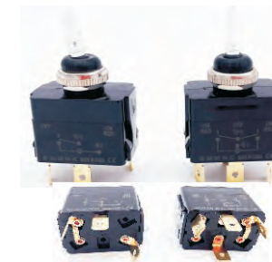
Plastic Toggle switch with Red led 12V 20A ; 24V 10A When On, red led lighting with waterproof boot nut SF CODE DETAILS SF50770S-1 ON-OFF , 3pin, SF50770S-2 (ON)-OFF , 3pin, SF50770S-3 On /Off /On, 4pin SF50770S-4 (On) /Off /On, 4pin SF50770S-5 (On) /Off /(On), 4pin
