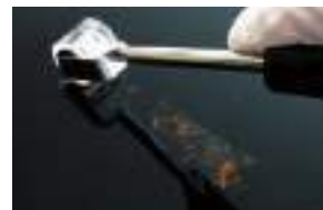
Transfer the dusts which removed by adhesive roller to Semiconductive gel sheet.
