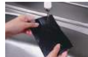
The adhesive power is restored by washing with water.
